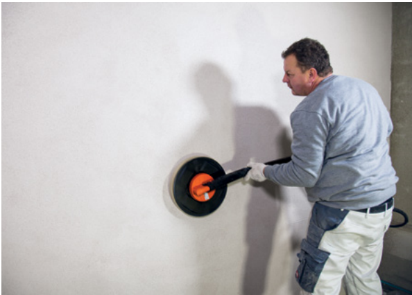
New engine technology: Lower rotation speed possible → for a perfect surface structure
