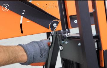
Remove the flat headed screw on the lefthand support bracket and remove the support bracket.
