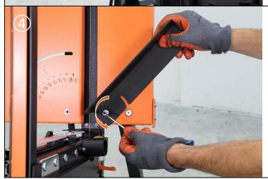
Remove the flat headed screw on the right-hand support bracket and remove the support bracket.
