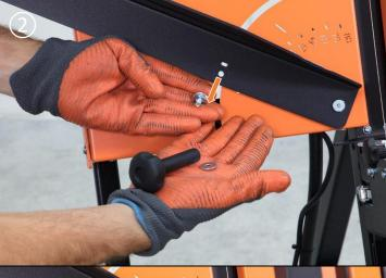
Remove the star knob including washers and guiding screw on the left support bracket.
